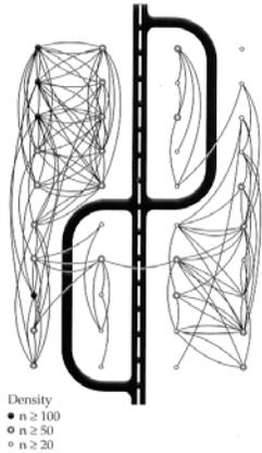
**Figure 7.13** Roads can be significant barriers to the movement of small vertebrates and invertebrates. In this example, populations of the forest-dwelling carabid beetle *Abax ater* were almost completely divided by a road and even by parking loops. Lines represent movements of marked beetles between capture and recapture points. (Modified from Mader 1984.)
